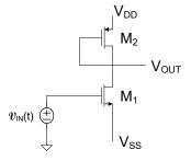
Problem 7 Design an amplifier using only MOS transistors, capacitors, and independent voltage sources that has a voltage gain of -10 when driving an external 10K resistor.
